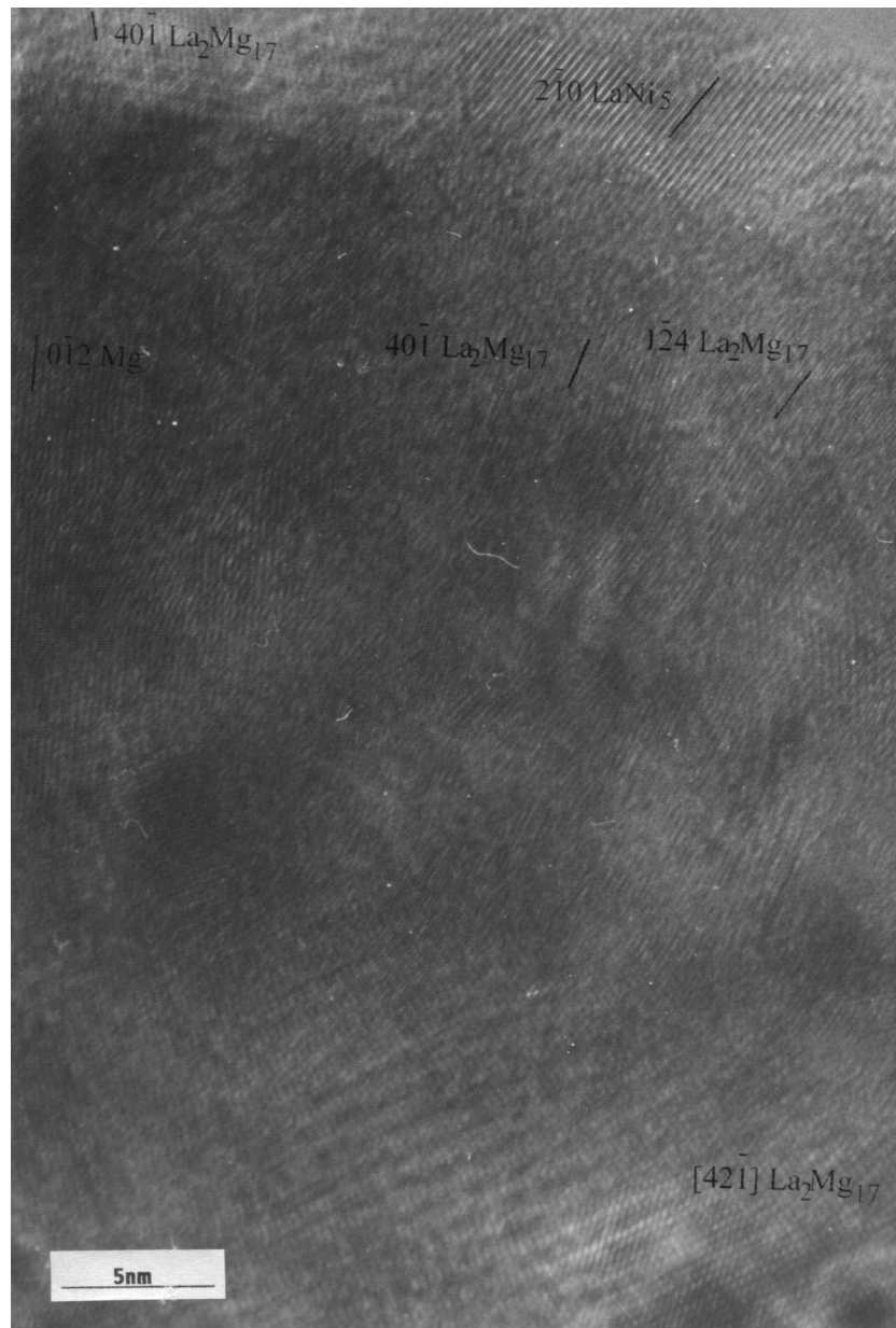
Fig. 5. HREM image of nano-phase composite alloys obtained by milling MmM_5 -30% Mg for 20 h.
